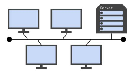
There is no need for a central hub like in physical star networks and a server can be connected to the backbone just like a client.
