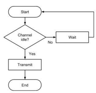
When a device is ready to transmit, it listens to its communication channel to check whether it is idle. If so, then the data is transmitted. If the channel is busy, the device waits for a random period of time before checking the channel again. An exponential backoff algorithm can be used to increase the time period for which the device waits with each check of the channel.
